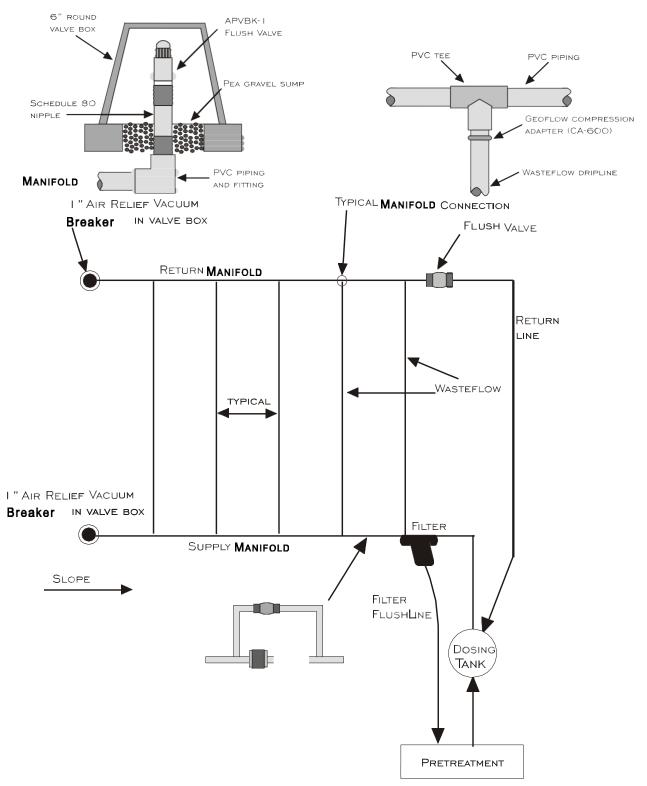
**Figure 2. Typical Drip Field Layout**
