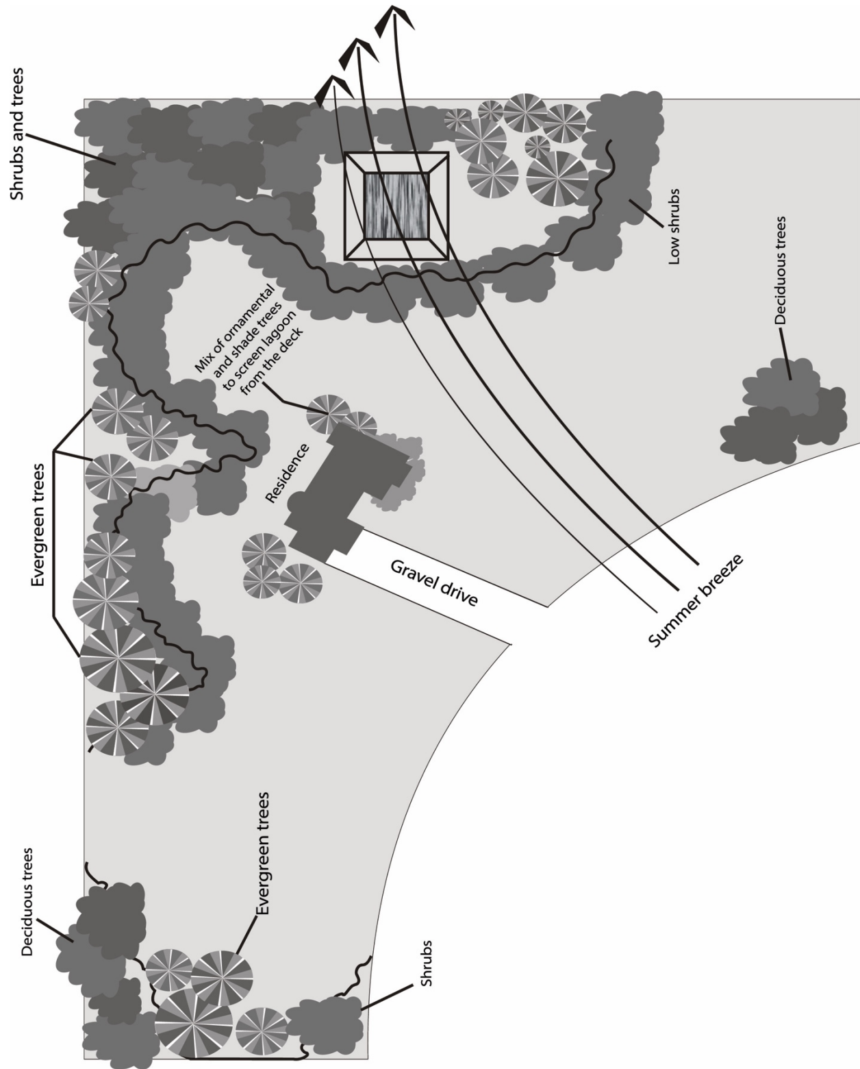
Figure IX-7. Lagoon Siting and Design
